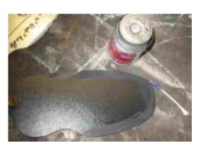
gloves because things are about to get hot. Fire up the heat gun and start moving the kydex through the heat zone. Try to get it as uniform as you can and don't over heat. I use a weak spring clamp as a handle when I do this. Keep waving the kydex through the heat until it becomes limp (probably about 200-250F) - or you could use a toaster oven. Once the material becomes about as stiff as thin leather, fold the edges together as shown here.
