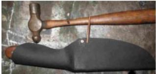
left over electrical wire (#12) makes quick and easy rivets. I use a rivet at the top and bottom of the seam.
